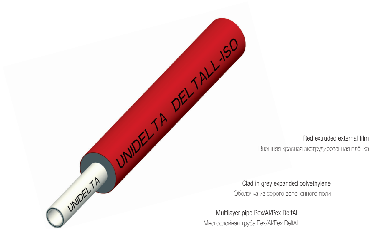
Fig.7.3 - The Structure Fig. 7.3 - La structure
